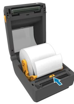
Align the sensor to the center of the roll for regular labels.
