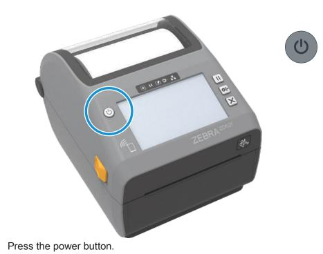
When the the printer is ready, the printer status light will turn green.
