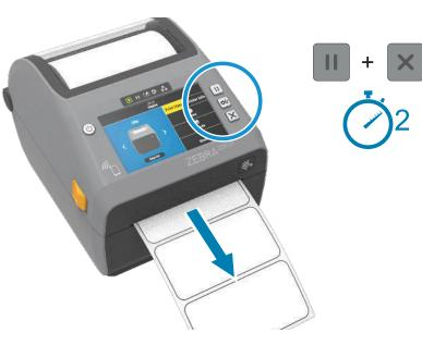
Press and hold the Pause and Cancel buttons for two seconds to line up the
