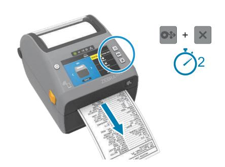
Press and hold the Feed and Cancel buttons for two seconds to print a configuration report.
