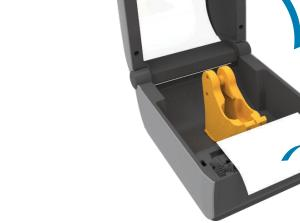
Open the printer and remove the packing.
